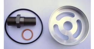
Ensure that the area around the oil filter housing is clean. Remove the old oil filter bowl and filter. Remove the central fixing boss and splash plate by inserting a tommy-bar through the holes in the boss and unscrewing in an anti-clockwise direction (it may be tight). Remove the old rubber seal from its groove in the oil pump / filter housing.
